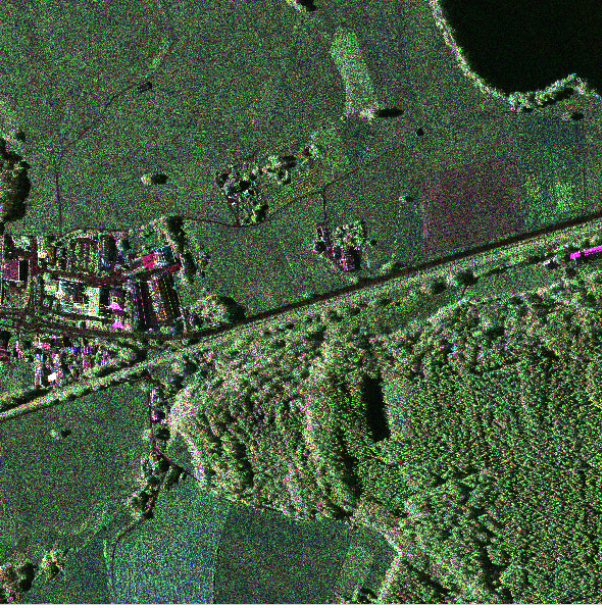
Fig. 1. Polarimetric FSAR X-band image with size 5000 \times 5000 pixels over Kaufbeuren site, Germany. The sensor used for this acquisition operates in the spectral X-band, has an altitude of 3045 meters and offers a pixel spacing of 15 centimeters in range and 17 centimeters in azimuth.
