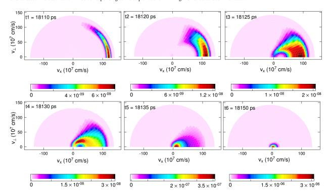
Figure 16: Distribution function of suprathermal  $\alpha$ -particles observed in the considered hot spot mesh  $i_0$  whose radius is represented in Fig. 15. The simulation takes into account the self-consistent modeling of creation, transport and collisional relaxation of  $\alpha$ -particles. Times refer to beginning of the implosion and the values of the distribution function are expressed in the units presented in table 1.
