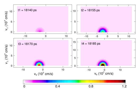
Figure 18: Thermal component of the  $\alpha$  distribution function observed he considered hot spot mesh  $i_0$  whose radius is represented on (Fig. 15). This thermal component is fed by the relaxation of the suprathermal component. The values of the distribution function are expressed in the units presented in table 1. Times refer to beginning of the implosion.
