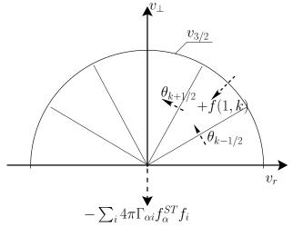
Figure 5: Central mesh of the suprathermal velocity grid
