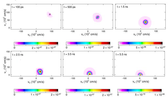
Figure 7:  $\alpha$  suprathermal distribution solution of the anisotropic test problem at different times. Final stages of collisional relaxation. The values of the distribution function are expressed in cgs units.
