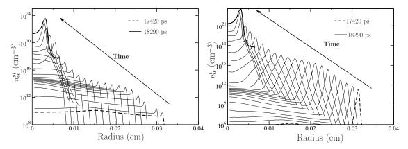
Figure 13: Density profiles of suprathermal (left) and thermal (right)  $\alpha$ -particles. The initial time (i) corresponds to t = 17.42 ns and the final time (f) to 18.29 ns. The time interval between two consecutive profiles is 36.67 ps.
