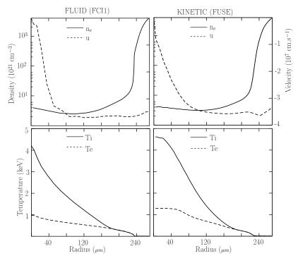
Figure 10: Comparison of the fluid(FCI1) and kinetic(Fuse) calculations. Profiles of the density, velocity and of the electron and total ion temperatures in a DT ignition target at the time t = 17.65 ns, which corresponds to 310 ps after the beginning of the kinetic calculation and roughly 650 ps before the target ignition.
