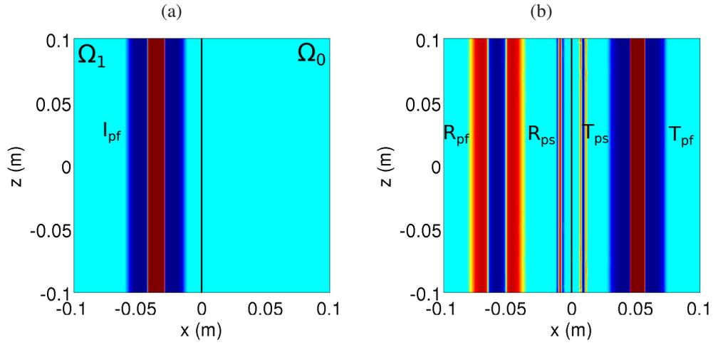
Figure 6: test 2. Snapshot of pressure at initial time (a) and at  $t_1 \approx 1.48 \cdot 10^{-5}$  s (b). The plane interface is denoted by a straight black line, separating  $\Omega_1$  (on the left) and  $\Omega_0$  (on the right).
