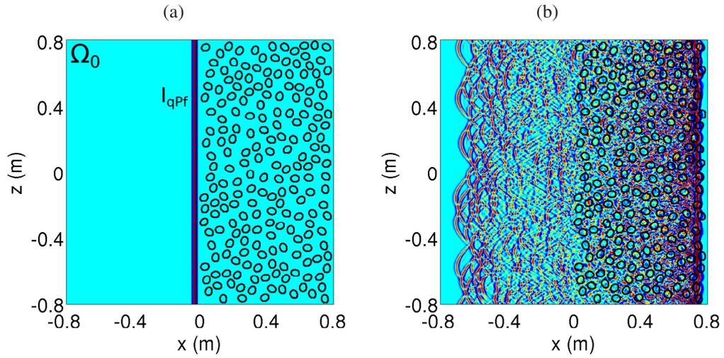
Figure 9: test 4. Multiple scattering in random media. Snapshot of  $p$  at the initial time (a) and at time  $t_1 \approx 1.43 \cdot 10^{-4}$  s. The matrix is  $\Omega_0$ , whereas the 200 scatterers are  $\Omega_1$ .
