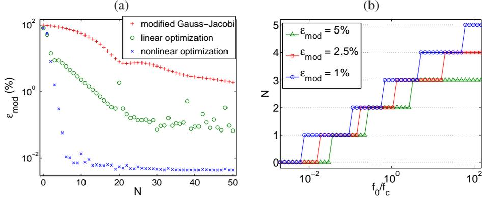
Figure 3: (a): relative error  $\varepsilon_{mod}$  in terms of  $N$  for both the modified Gauss-Jacobi quadrature and the nonlinear constrained optimization. (b): required values of  $N$  in terms of  $f_0/f_{c1}$  and the required accuracy  $\varepsilon_{mod}$  for the nonlinear optimization.
