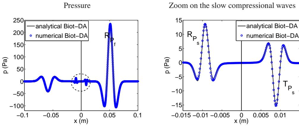
Figure 7: test 2. Pressure along the line  $z = 0$  m; vertical line denotes the interface. Comparison between the numerical values (circle) and the analytical values (solid line) of  $p$  at  $t_1 \approx 1.48 \cdot 10^{-5}$  s.
