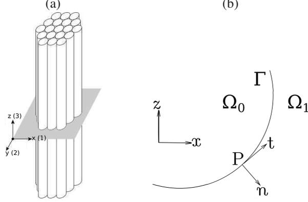
Figure 1: medium under study. (a): the physical properties are symmetric about the axis  $z$  that is normal to the plane  $(x, y)$  of isotropy. (b): interface  $\Gamma$  separating two poroelastic media  $\Omega_0$  and  $\Omega_1$ . The normal and tangential vectors at a point  $P$  along  $\Gamma$  are denoted by  $\mathbf{n}$  and  $\mathbf{t}$ , respectively.
