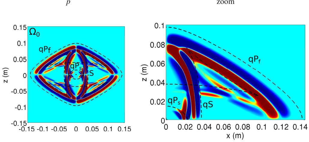
Figure 5: test 1. Fast and slow quasi-compressional waves, respectively  $qP_f$  and  $qP_s$ , and quasi-shear wave  $qS$  emitted by a source point at  $(0 \text{ m}, 0 \text{ m})$ . Pressure at  $t_1 \approx 2.72 \cdot 10^{-5} \text{ s}$ .
