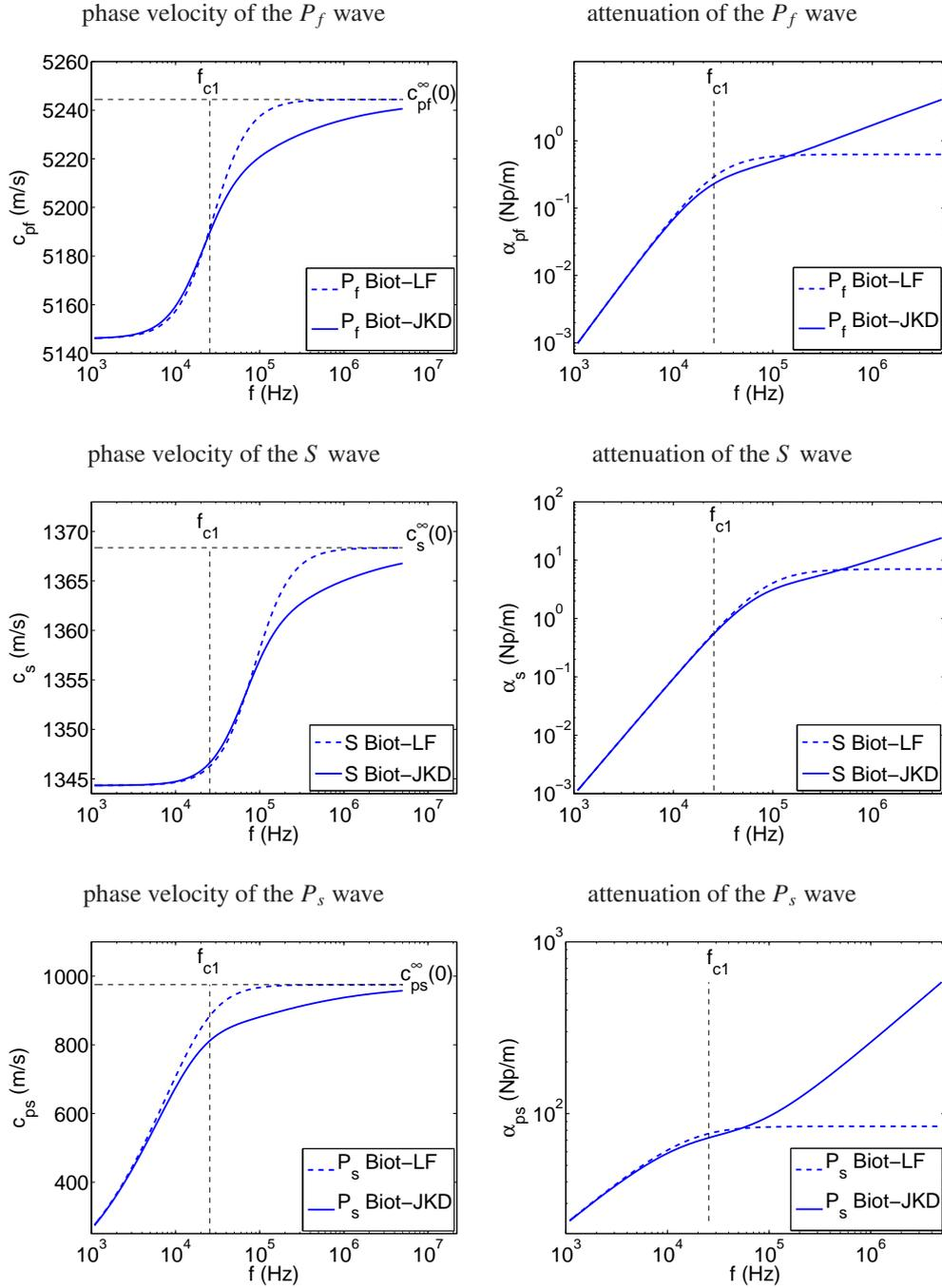
Figure 2: dispersion curves in terms of the frequency. Comparison between Biot-LF and Biot-JKD models at  $\varphi = 0$  rad. The vertical dotted line denotes the critical frequency separating low-frequency and high frequency regimes. The horizontal dotted lines in the left row denote the maximal phase velocity at infinite frequency.
