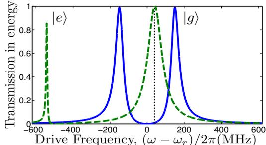
FIG. 2: Transmission coefficient at low pump power for a microwave pulse injected in a resonator containing a diamond-shape artificial atom. Blue solid curve: Qubit state  $|g\rangle$ . Green dashed curve: Qubit state  $|e\rangle$ . Frequency is centered on the bare cavity. We took  $g_{zz}/2\pi = 250$  MHz,  $g_a/2\pi = 150$  MHz and a cavity linewidth  $\kappa/2\pi = 40$  MHz ( $Q = 250$ ) and  $p \ll p_s$ . The black dotted line indicates the pump frequency  $\omega$ .
