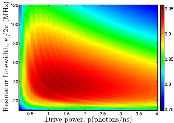
FIG. 4: Single measurement fidelity for a state of the art amplifier ( $T_N = 140\text{mK}$ ) and an acquisition time  $\tau = 10\text{ns}$  versus drive power  $p$  in units of photons/10ns and resonator linewidth  $\kappa$ . Optimal value of  $\mathcal{F} = 95\%$  is reached for broad range around  $\kappa = 40\text{MHz}$  and  $p = 1\text{photon/ns}$ .
