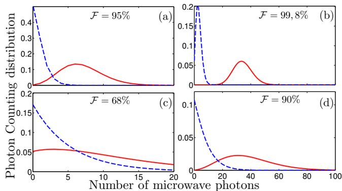
FIG. 3: Photon distribution at the entrance of the amplifier. Histograms  $\mathbf{P}(n|e)$  (red solid) and  $\mathbf{P}(n|g)$  (blue dashed) with  $\kappa = 40\text{MHz}$  and  $p = 1\text{photon/ns}$ . (a)  $T_N = 140\text{mK}$ ,  $\tau = 10\text{ns}$ ,  $B = 50\text{MHz}$ ; (b)  $T_N = 140\text{mK}$ ,  $\tau = 50\text{ns}$ ,  $B = 10\text{MHz}$ ; (c)  $T_N = 4\text{K}$ ,  $\tau = 10\text{ns}$ ,  $B = 50\text{MHz}$ ; (d)  $T_N = 4\text{K}$ ,  $\tau = 50\text{ns}$ ,  $B = 10\text{MHz}$
