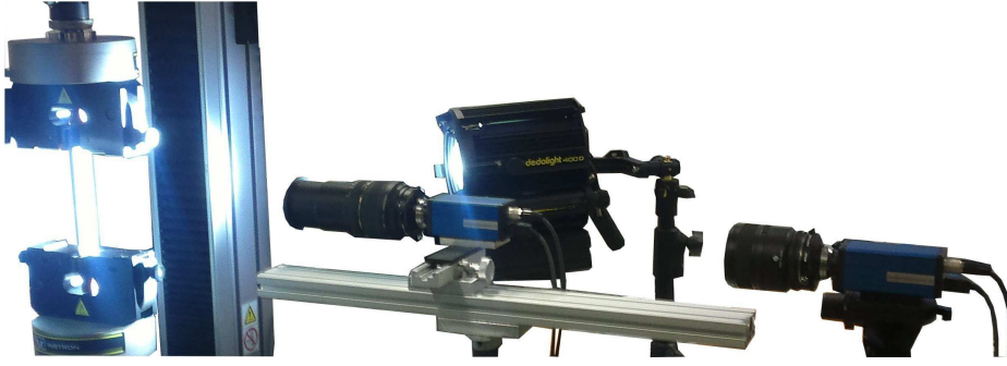
Fig. 8 Experimental setup. The two digital cameras are facing the specimen: their optical axis is perpendicular to the laminate plane. Here, a translation stage is used to retract the nearfield camera in order to capture the farfield image.
