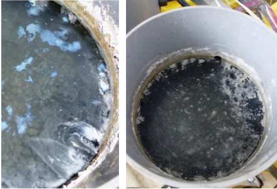
Figure 5 Outflow of the UF-GU column with visible white precipitates
