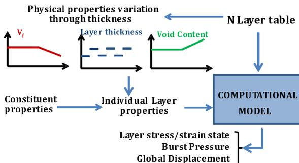
Figure 3. Thick composites pressure vessel design model
