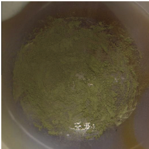
Fig. 5. Final product after the complete chlorination procedure (green sticky powder). (For interpretation of the references to colour in this figure legend, the reader is referred to the web version of this article.)
