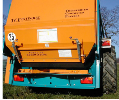
Photo 2. Spreader with spreading table
