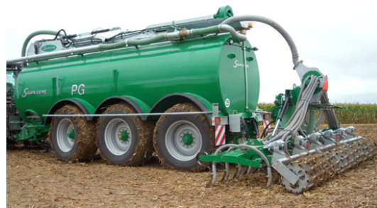
Photo 4. High capacity tanker with injectors
