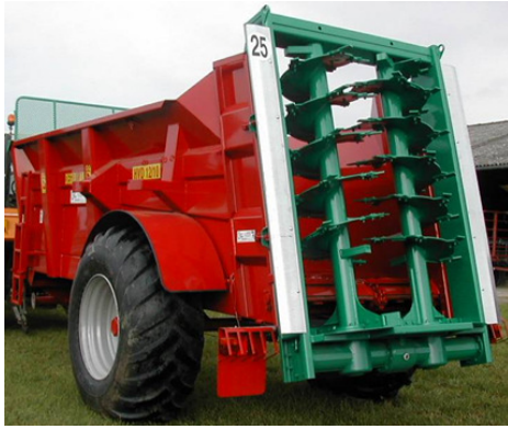
Photo 1. Spreaders with two vertical rotors
