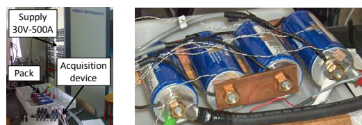
(a) Test bench (b) supercapacitors of one pack Fig. 1: Photo of the test bench
