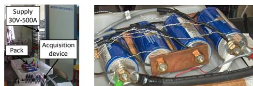
(a) Test bench (b) supercapacitors of one pack
