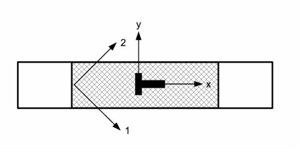
Figure 1: Schematic view of the classical tensile test coupon with longitudinal and transverse strain gauges (in black). In the present case  $a \pm 45^{\circ}$  configuration is depicted.
