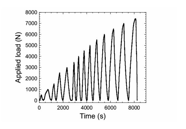
Figure 3: Applied load (N) versus time (s). Each local peak data were used to measure displacement fields by resorting to DIC.
