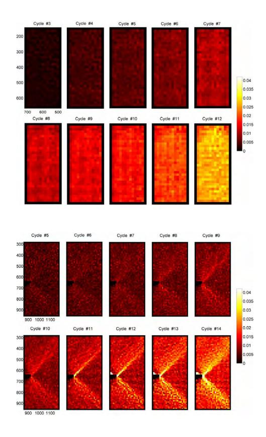
Figure 7: Equivalent (shear) strain maps for each step up to failure in a tensile test for the classical geometry (top: cycles #3 to #12) with a 16-pixel discretization, and for a notched sample (bottom: cycles #5 to #14) with a 12-pixel discretization.
