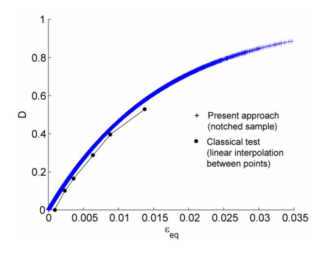
Figure 11: Damage law identified by following the classical approach (few strain data are available) and by resorting to full-field measurements and the equilibrium gap method. Each cross corresponds to a measured strain.
