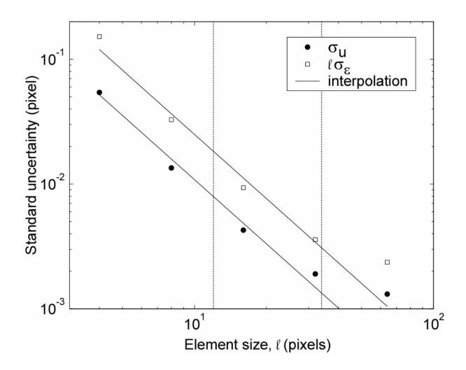
Figure 6: A priori analysis of the standard displacement  $(\sigma_u)$  and strain  $(\sigma_\epsilon)$  uncertainties as functions of the element size  $(\ell)$  for the reference picture of the analyzed experiment. The symbols are measurement results and the solid lines correspond to a power law fit.
