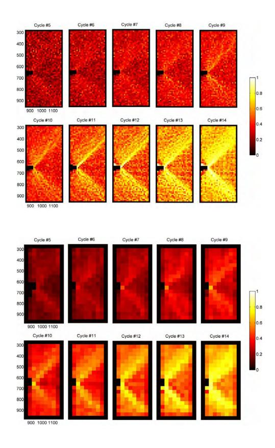
Figure 9: Identified damage maps for each analyzed cycle for two elements sizes: 12 pixels (top), and 34 pixels (bottom).
