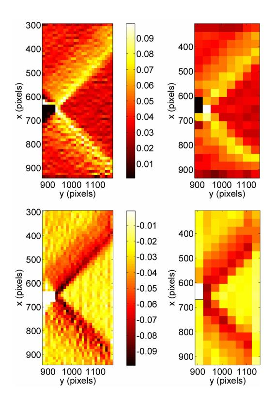
Figure 5: Strain maps  $\varepsilon_{xx}$  (top) and  $\varepsilon_{yy}$  (bottom) at last step of the analysis of the notched specimen with a 12-pixel (left) and 34-pixel (right) discretization. Strain localization (along the fiber directions) is clearly visible on both maps of the finer discretization.
