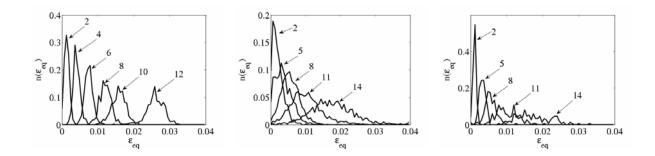
Figure 8: Probability density functions of equivalent strains in the classical geometry with a 16-pixel discretization (left), and in the notched specimen with 12-pixel (middle) and 34-pixel (right) discretizations. Each curve corresponds to one cycle.
