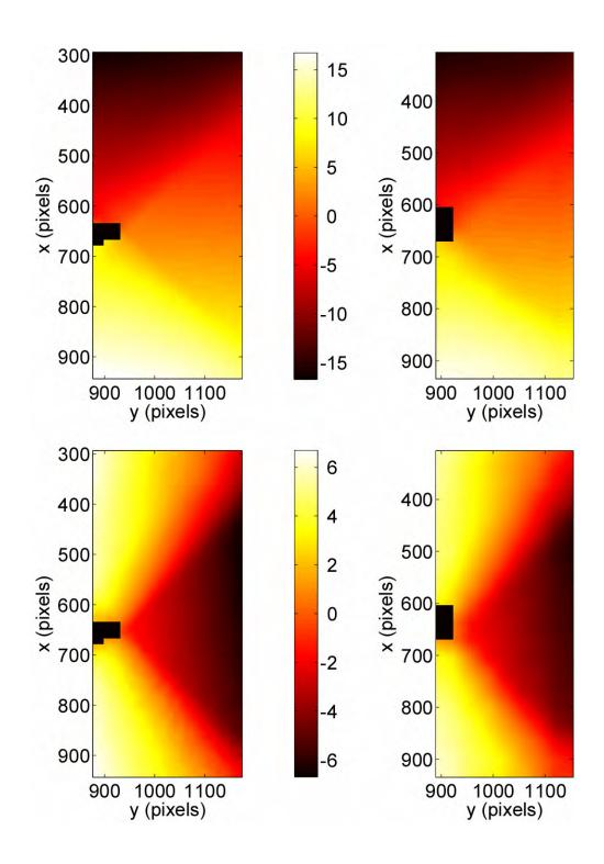
Figure 4: Displacement maps  $u_x$  (top) and  $u_y$  (bottom) expressed in pixels (1 pixel  $\leftrightarrow$  36  $\mu$ m) at maximum load of the notched specimen with a 12-pixel (left) and 34-pixel (right) discretization. The rigid body motion was removed.
