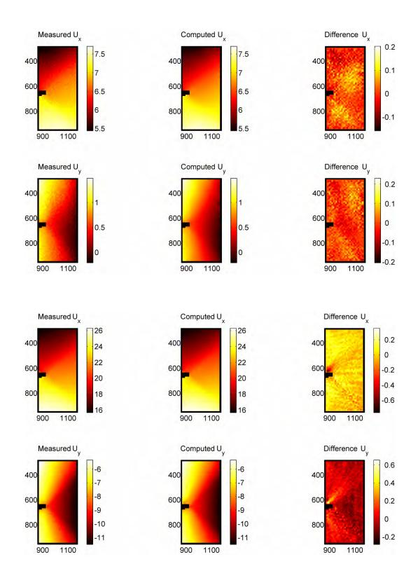
Figure 10: Comparison of the measured and computed displacement fields (top: cycle #4, bottom: cycle #14) for the 12-pixel discretization.
