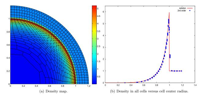
Figure 11: Second-order DG scheme with limitation; Numerical results for the Sedov problem on a polygonal grid made of 775 polygonal cells.
