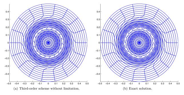
Figure 19: Gresho problem variant on a polar grid made of  $40 \times 18$  cells at the final time t = 1. Grid deformations obtained with the third-order scheme without limitation and the analytical solution.
