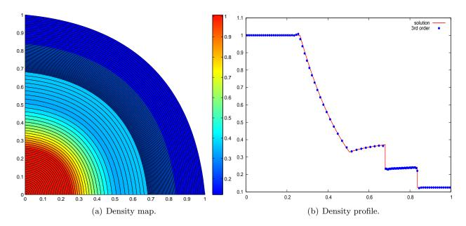
Figure 16: Polar Sod shock tube problem. Solution obtained with the third-order DG scheme without limitation on the domain defined in polar coordinates by  $(r, \theta) \in [0, 1] \times [0, \frac{\pi}{2}]$  made of  $100 \times 1$  cells.
