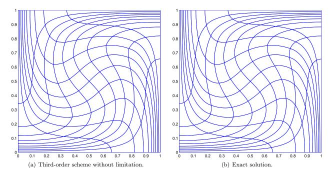
Figure 22: Taylor-Green vortex deformation of a Cartesian grid made of  $10 \times 10$  cells, at time t = 0.75.
