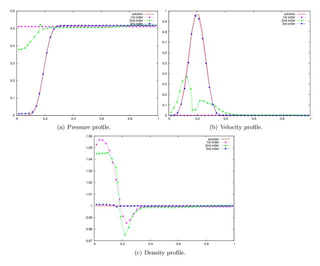
Figure 20: Gresho problem variant on a polar grid made of  $40 \times 18$  cells at the final time t = 1: comparison between the analytical solution and those obtained with the first, second and third-order numerical schemes, plotted at the centroid of the cells.
