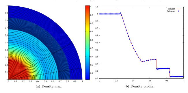
Figure 15: Polar Sod shock tube problem. Solution obtained with the third-order DG scheme without limitation on the domain defined in polar coordinates by  $(r, \theta) \in [0, 1] \times [0, \frac{\pi}{2}]$  made of  $100 \times 3$  non-uniform cells.
