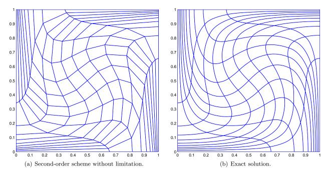
Figure 12: Taylor-Green vortex deformation of a Cartesian grid made of  $10 \times 10$  cells, at time t = 0.75.
