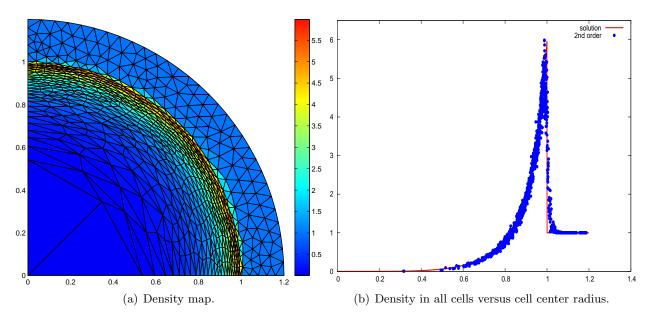
Figure 10: Second-order DG scheme with limitation; Numerical results for the Sedov problem on a triangular grid made of 1110 cells.
