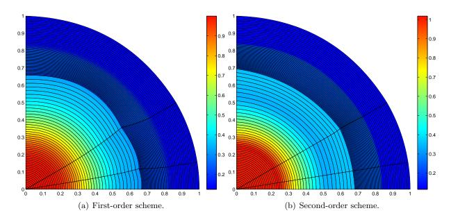
Figure 14: Polar Sod shock tube problem. Density maps obtained with the first and second-order DG schemes on the domain defined in polar coordinates by  $(r, \theta) \in [0, 1] \times [0, \frac{\pi}{2}]$  made of  $100 \times 3$  non-uniform cells.
