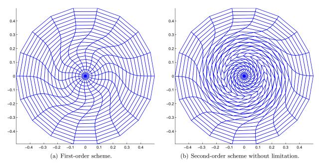
Figure 18: Gresho problem variant on a polar grid made of  $40 \times 18$  cells at the final time t = 1. Grid deformations obtained with the first and second order scheme.
