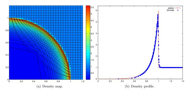
Figure 21: Point blast Sedov problem on a Cartesian grid made of  $30 \times 30$  cells with the third-order scheme with limitation.
