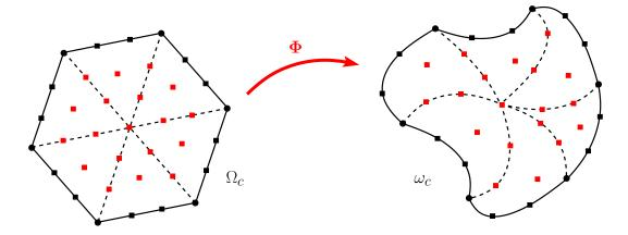
Figure 5: Transformation of  $\Omega_c$  to  $\omega_c$  through the flow. • boundary cell nodes,  $\blacksquare$  boundary cell control points,  $\blacksquare$  interior cell points.
