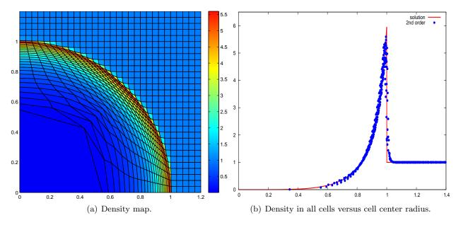
Figure 8: Second-order DG scheme with limitation; Numerical results for the Sedov problem on a  $30 \times 30$  Cartesian grid.
