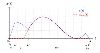
Figure 2: An example of a MIO policy for T=10,  $\lambda(t)=2(1-\cos(\frac{t}{2}))$ ,  $\mu(t)=2.5$ . Time intervals  $a_1$  and  $a_2$  correspond to production (active) periods while  $i_1$  and  $i_2$  are idle periods.
