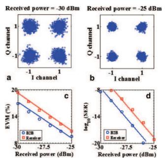
Fig. 13 Constellation diagrams (a-b) and RoF system performance illustrated through the corresponding error vector magnitude (c) and symbol error ratio (d) plots
