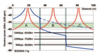
Fig. 1 Received power (in decibel-milliwatt) with distance (in metre) in the case of distributed antennas vs. single antenna systems
