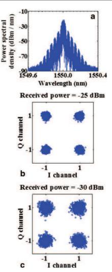
Fig. 10 Optical spectrum (a) and constellation diagrams (b)–(c) of the 10-Gbps QPSK signal transmitted at the downlink
