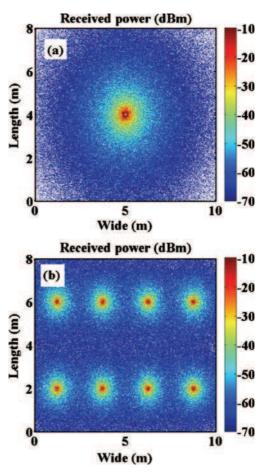
**Fig. 7** Received power (in decibel-milliwatt) by a mm-wave terminal operating under the IEEE Standard 802.15.3c, considering a single access point with a total radiated power of 13 dBm (**a**) and an eight-antenna system with a total radiated power of 9 dBm (**b**)
