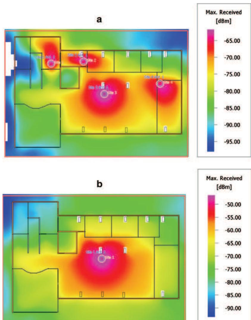
**Fig. 4** Simulated wireless coverage ( $P_r$  level) of a 60-GHz foam antenna for different positions in the horizontal plane ( $x, y$ ) and different values of the tilt angle (from the ceiling plane): 45° (a), 25° (b), 30° (c)
