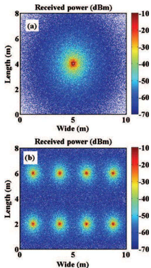
**Fig. 7** Received power (in decibel-milliwatt) by a mm-wave terminal operating under the IEEE Standard 802.15.3c, considering a single access point with a total radiated power of 13 dBm (a) and an eight-antenna system with a total radiated power of 9 dBm (b)
