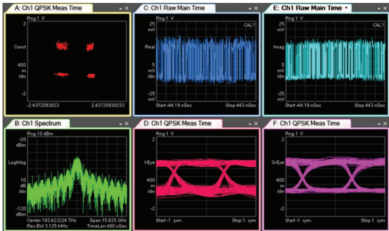
**Fig. 14** Optical spectrum and constellation diagram of a QPSK optical signal at 5 Gbaud recorded by an optical coherent receiver for an input power of  $-5$  dBm. Time domain traces and eye diagrams of the in-phase and quadrature channels are also illustrated
