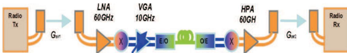
**Fig. 5** The system architecture of the ORIGIN demonstrator. Point-to-point variant. Orange parts work at 60 GHz, blue parts at the intermediate frequency and green parts are optical components
