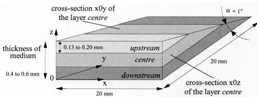
Figure 2. Schematic view of consolidated sample slices.
