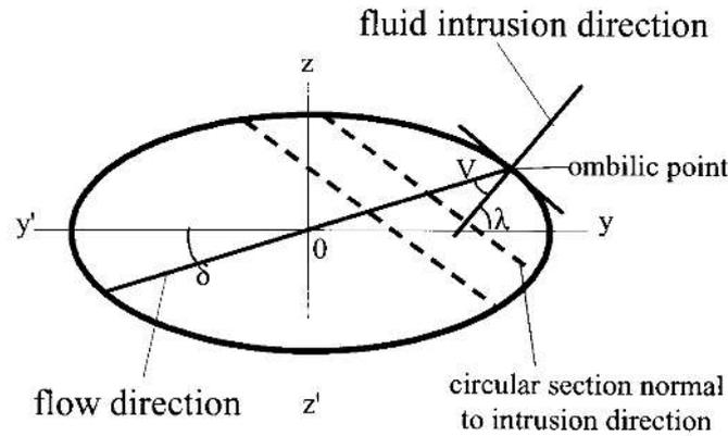
Figure 1. Representation of the equivalent pore model [7].
