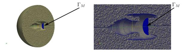
Figure 9: Cut of the mesh of the simplified engine.
