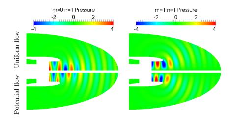
Figure 12: Simplified engine: comparison of the pressure for the uniform model  $(M_{\infty} = M_M = 0.3)$ and the potential model  $(M_{\infty} = 0.3 \text{ and } M_M = 0.42)$ .
