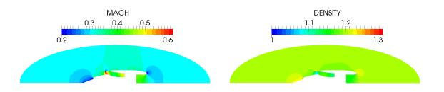
Figure 10: Simplified engine: computed potential flow such that  $M_M = 0.42$  and  $M_{\infty} = 0.3$  (*left*: Mach number, *right*: density).
