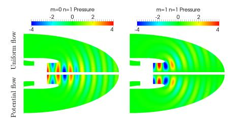
Figure 11: Simplified engine: comparison of the pressure for the uniform model and the potential model with  $M_{\infty} = M_M = 0.3$ .
