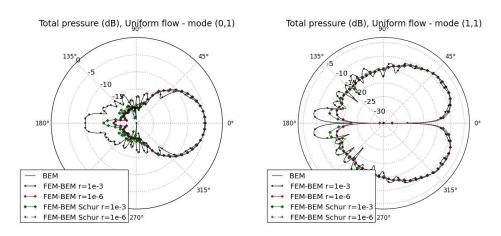
Figure 14: Simplified engine: influence of the convergence criteria and on the pressure in dB on a circle at r = 20 m for an uniform flow defined by  $M_M = M_{\infty} = 0.1$ .
