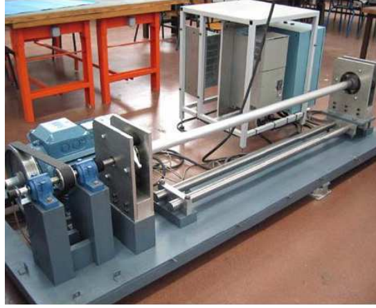
Fig. 5. Testing machine for high-speed tubes
