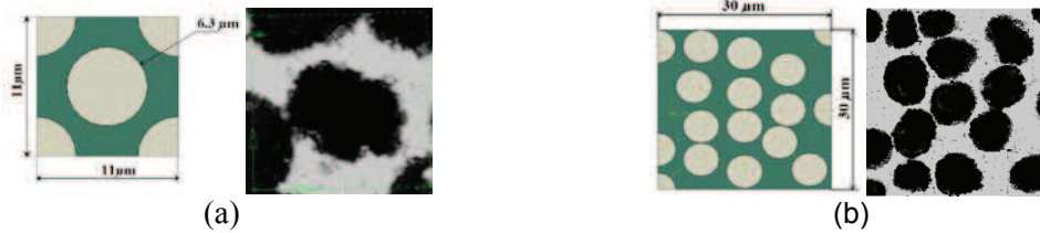
Figure 3: The periodic representative elementary volume of the yarn, number of fiber N = 2 fibers (a) and v_f = 0.505 . The random representative elementary volume of the yarn, number of fiber N = 14 fibers and v_f = 0.475 (b)
