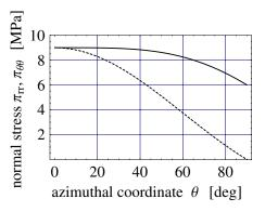
Fig. 2 Effect of edge boundary condition—profile of radial and azimuthal normal stress. Azimuthal normal stress equals ambient pressure at film edge. Simple steady squeezing flow  $\epsilon$  =0.0. Relaxation time  $\lambda$ =1 s; PTT parameter  $\xi^*$ =0.0 (Maxwell fluid). Dashed line: normal stress in flow direction  $\pi_{\theta\theta^*}$  Solid line: load carrying normal stress  $\pi_{rr}$ .
