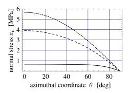
Fig. 3 Effect of relaxation time—profile of radial (load carrying) normal stress. Simple squeezing flow  $\epsilon$ =0.0. PTT parameter  $\xi^*$ =0.1. Solid line:  $\lambda$ =1 s; long dashed line:  $\lambda$ =0.5 s; short dashed line: Newtonian,  $\lambda$ =0.0 s.
