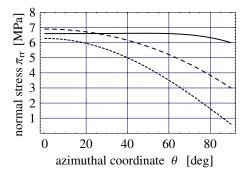
Fig. 4 Effect of relaxation time—profile of radial (load carrying) normal stress. Normal stress  $\pi_{\theta\theta}$  set to ambient at film edge. Simple squeezing flow  $\epsilon$ =0.0. PTT parameter  $\xi^{*}$ =0.1. Solid line:  $\lambda$ =1 s; long dashed line:  $\lambda$ =0.5 s; short dashed line:  $\lambda$ =0.1 s.
