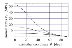
Fig. 6 Effect of eccentricity—profile of radial (load carrying) normal stress. Simple squeezing flow. Relaxation time  $\lambda$  =0.1 s. PTT parameter  $\xi$ \*=0.1. Solid line:  $\epsilon$ =0.0; short dashed line:  $\epsilon$ =0.5; long dashed line:  $\epsilon$ =0.8.
