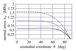
Fig. 5 Effect of PTT shear parameter  $\xi$ —profile of radial (load carrying) normal stress. Simple squeezing flow  $\epsilon$ =0.0. Relaxation time  $\lambda$ =1 s. Solid line:  $\xi$ \*=0.1; short dashed line:  $\xi$ \*=0.08; long dashed line:  $\xi$ \*=0.05.
