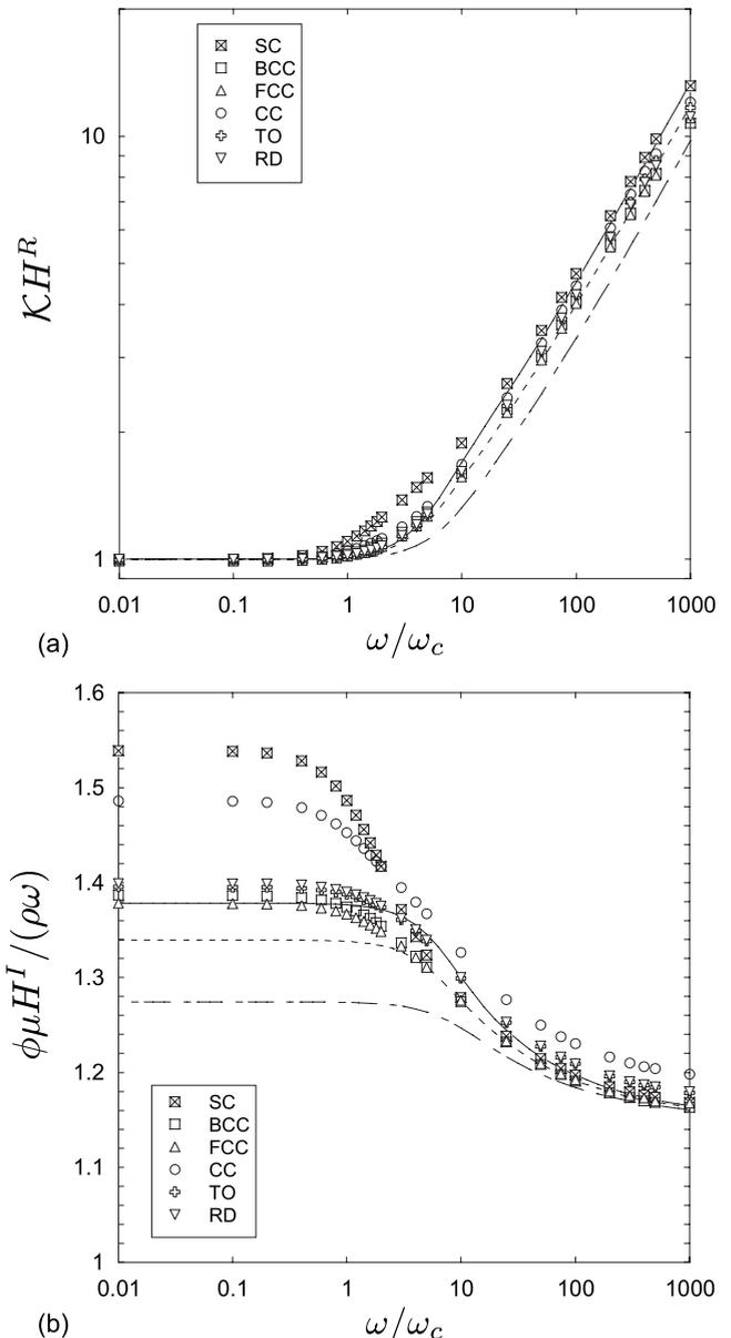
FIG. 10. Dimensionless real and imaginary part of  $\mathbf{H}$  versus  $\omega/\omega_c$  when the porosity  $\phi=0.7$ . Comparison between estimates: P-estimate (continuous line), C-estimate (dashed line), V-estimate (mixed line) and numerical results for the different packings of spheres and polyhedrons (marks).
