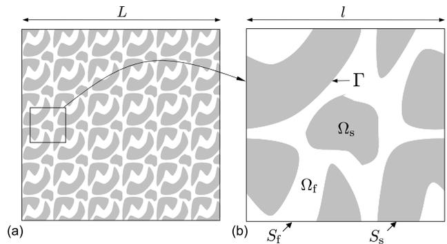
FIG. 1. (a) Macroscopic porous medium, (b) Periodic cell  $\Omega$  of porous media.  $\Omega_f$  and  $\Omega_s$  are respectively the volume of fluid and solid.  $\Gamma$  is the fluid-solid interface inside  $\Omega$ .  $S_f$  and  $S_s$  are the fluid and the solid boundaries on  $\partial\Omega$ .
