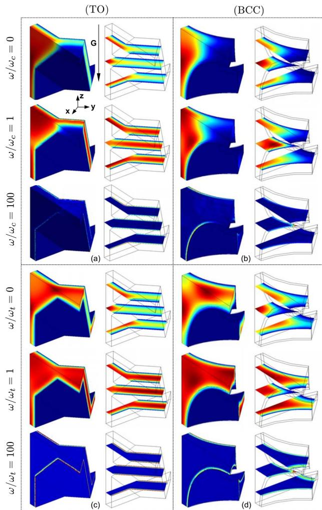
FIG. 9. (Color online) Color on line. Influence of the ratio  $\omega/\omega_c$  (resp.  $\omega/\omega_t$ ) on the microscopic velocity field  $\mathbf{v}^0$  (respectively, the local temperature field  $T^0$ ) when the porosity  $\phi=0.25$  in packing of polyhedrons (a) [respectively, (c)] and spheres (b) [respectively, (d)]. The intensity varies between 0 (in blue) and a maximum value (in red).
