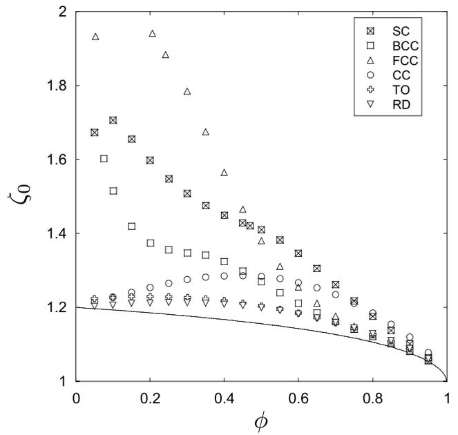
FIG. 13. Corrector for the low-frequency heat capacity  $\zeta_0$  versus porosity  $\phi$ . Comparison between estimate  $\zeta_{sc0}$  (continuous line) and numerical results for the different packings of spheres and polyhedrons (marks).
