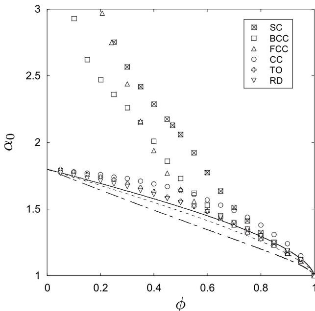
FIG. 6. Evolution of low-frequency tortuosity  $\alpha_0$  versus the porosity  $\phi$ . Comparison between estimates:  $\alpha_{0p}$  (continuous line),  $\alpha_{0c}$  (dashed line),  $\alpha_{0v}$  (mixed line) and numerical results for the different packing of spheres and polyhedrons (marks).
