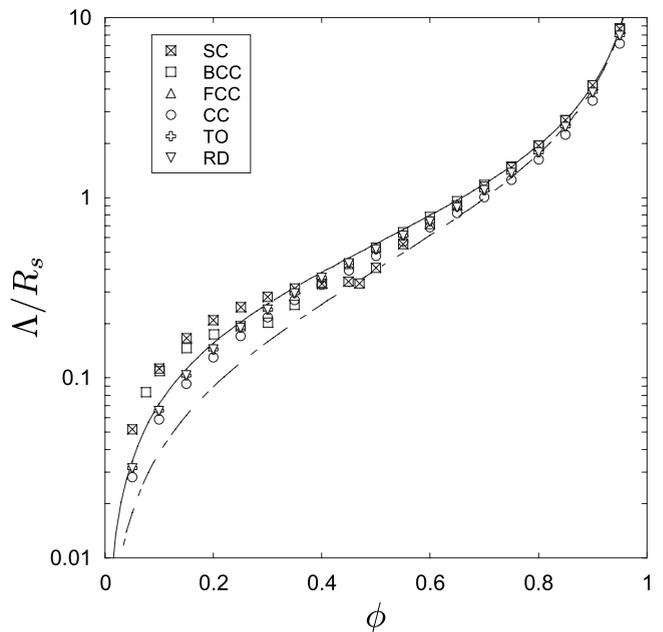
FIG. 8. Dimensionless viscous length  $\Lambda/R_s$  versus porosity  $\phi$ . Comparison between estimates:  $\Lambda_p$  (continuous line),  $\Lambda_v$  (mixed line) and numerical results for the different packings of spheres and polyhedrons (marks).
