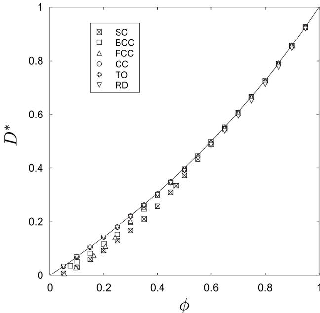
FIG. 4. Dimensionless effective diffusion coefficient  $D^* = \tilde{D}/D$  versus porosity  $\phi$ . Comparison between self-consistent estimate [Eq. (13)] (continuous line) and numerical results for the different packings of spheres and polyhedrons (marks).
