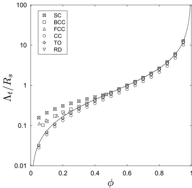
FIG. 15. Dimensionless viscous layer thickness  $\Lambda_t/R_s$  versus porosity  $\phi$ . Comparison between estimate  $\Lambda_{isc}$  (continuous line) and numerical results for the different packings of spheres and polyhedrons (marks).
