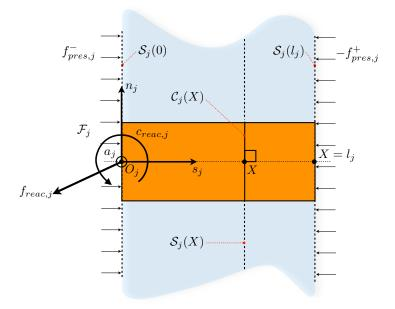
Figure 4: Schematic view of the fluid laterally surrounding a robot segment (i.e. when j is even).
