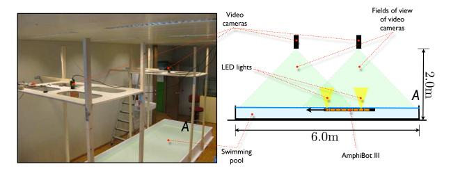
Figure 6: From the left to the right, a global view of the experimental setup and a schematic view of the measurement process.
