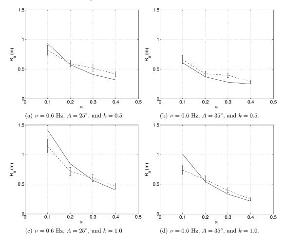
Figure 11: Steady state turning manoeuvre: The radius of the robot trajectory  $R_a$  is plotted as a function of the turning parameter  $\alpha$  for the four desired shape motions defined in table 2. Dashed line: experimental results. Continuous line: simulation results. The vertical error bars indicate the standard deviation of experimental measurements.
