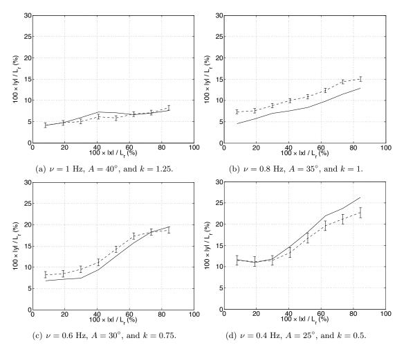
Figure 9: Forward swimming in a straight line: Maximal lateral displacements  $(100 \times |x|/L_r)$  of segments along the body  $(100 \times |y|/L_r)$  measured with respect to the forward direction of swimming (dashed lines: robot; continuous lines: simulator;  $L_r$  = robot length). The vertical error bars show the standard deviation of experimental measurements.
