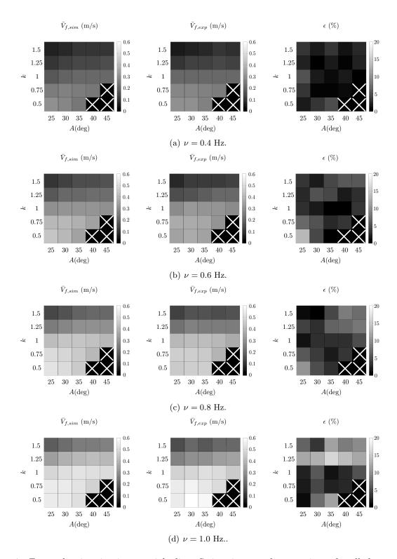
Figure 7: Forward swimming in a straight line: Swimming speed comparisons for all the tested forward swimming gaits as function of  $\nu$ , A and k. The left, middle and right columns represent, from  $\nu=0.4$  Hz (top row) to  $\nu=1.0$  Hz (bottom row), the numerical results, the experimental results and the relative errors respectively. The white crosses represent the unstable gaits for which the speed could not be estimated.
