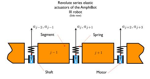
Figure 2: The series elastic actuators of the AmphiBot III.
