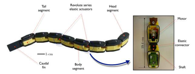
Figure 1: From the left to the right, a global view of the snake-like robot AmphiBot III and an internal view of two robot segments.
