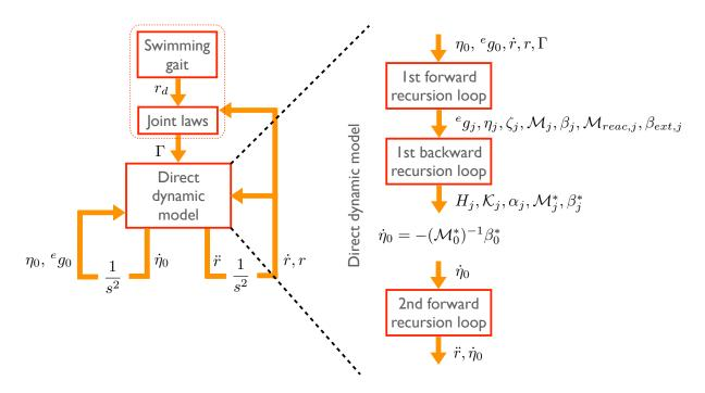
Figure 5: Schematic view of the direct dynamic model (DDM). The DDM computes the head segment accelerations and joint accelerations as a function of torques  $\Gamma$ , hydrodynamic forces  $F_{ext}$  and the head state ( ${}^{e}g_{0}$ ,  $\eta_{0}$ ).
