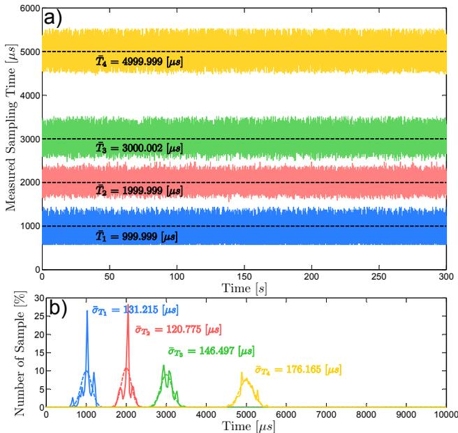
Fig. 8. a) The measured sampling time of the different tasks over the time. The sampling time is well respected by the embedded Linux and the maximum delay measured is about 400  $\mu\text{s}$ . The mean sampling time is really accurate as it differs only of 0.1% with respect to the targeted sampling time. b) The distribution of measured sampling time. The standard deviation is relatively small allowing to reach good timing performances up to 1kHz.
