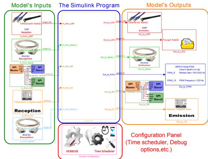
Fig. 2. Overview of the RT-MaG blockset. This example is composed of one wifi connexion (reception and emission), two serial ports (reception and emission), one SPI bus (reception and emission), one output to a log file, and two PWM outputs. The Simulink program is encapsulated in a sub-system block and all the configuration options are set via a specific block.
