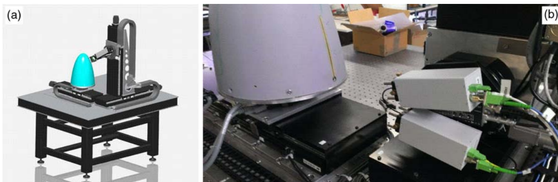
Fig. 1 The DOTNAC three-dimensional (3-D) scanner platform; schematic drawing with mounted FMCW sensor head (a), photograph of mounted TDS sensor and test radome (b).
