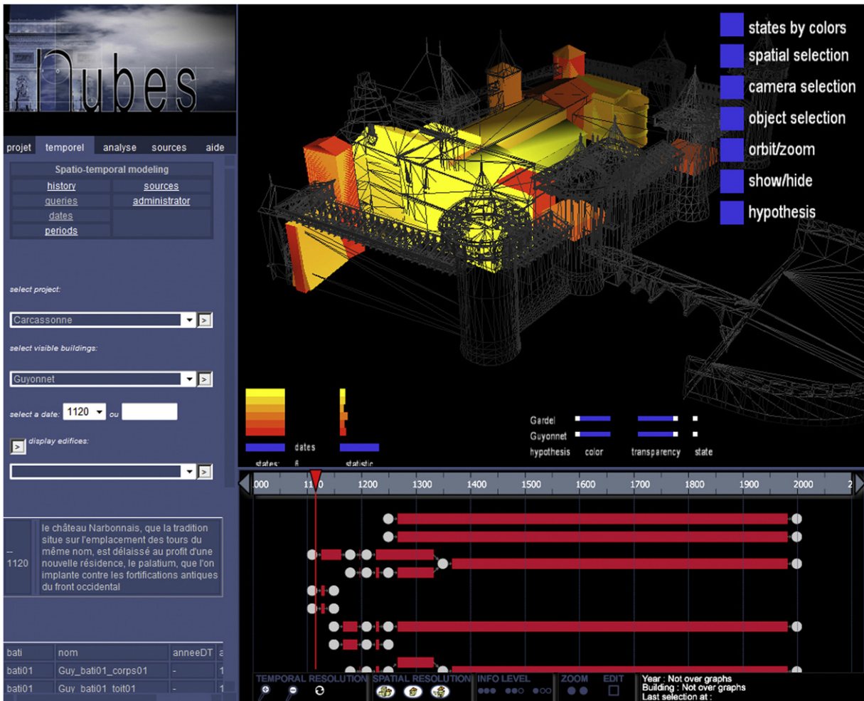
Fig. 9. Semantic-based temporal query interface. In this visualization system, the user can formulate temporal queries (left), display buildings according to their ancientness, isolate and compare assumptions (top) and display transformations by means of historic graphs (bottom). When a 3D element is selected, its history is displayed and vice versa, at the graph selection, the corresponding 3D elements are displayed.
