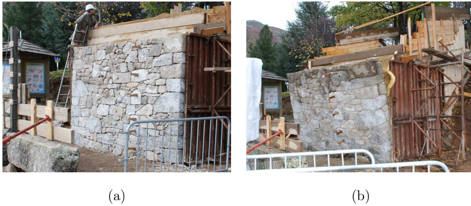
Figure 8: Full-scale field trials of dry-stone walls: preparation before experimentation (a) and overturning of the wall (b).
