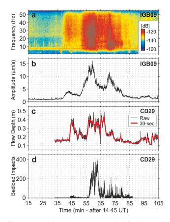
**Figure 9.** Flow pulse characteristics on the distal fan. (**a**) Spectrogram in decibel of the vertical seismic signal at station IGB09 during passage of flow pulses 1–3. (**b**) [5–50] Hz vertical seismic envelop at IGB09 showing three flow pulses. (**c**) Raw (black line) and 30 s smoothed (red line) flow depth data recorded at CD29, 400 m downstream of IGB09 (2 min at established flow speed). (**d**) Bedload impact rates recorded at CD29.
