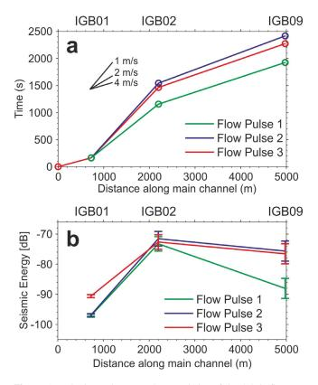
**Figure 8.** Velocity and energy characteristics of the debris flow sequence. (a) Downstream propagation of the three main flow pulses. The propagation is defined with the recordings of seismic envelopes at side-stream stations IGB01, IGB02 and IGB09. (b) Mean seismic energy of each flow pulse recorded at the same stations. The amplitude in decibel is corrected for the geometrical spreading of body waves.
