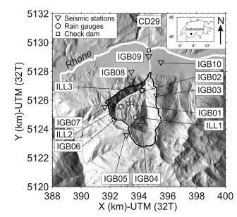
**Figure 1.** The Illgraben catchment. Location of the Illgraben catchment ( $\sim 10 \text{ km}^2$ , outlined in black) in Switzerland (dot in the inset map) and of the seismological stations deployed there during summer 2011 (inverse triangles, labelled IGBnn), meteorological stations from the Swiss Federal Institute for Forest, Snow and Landscape Research WSL (circles, labelled ILLn), and check dam 29 (CD29, square) where the flow depth and bedload impact rates of the study were observed.
