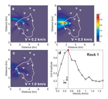
**Figure 5.** Location of mass wasting events in the Illgraben. (**a**–**c**) Probability density map (unit amplitude) for rock 1 location in the [29–29.5] Hz frequency band. Migration velocities are 0.2 (**a**), 0.5 (**b**) and  $1.0 \text{ km s}^{-1}$  (**c**). (**d**) Migration velocity analysis where the maximum amplitude corresponds to the best fit propagation velocity (0.5 km s<sup>-1</sup> for rock 1).
