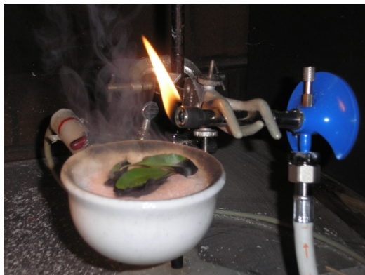
Fig. 3 Epiradiator used in the flammability experiments
