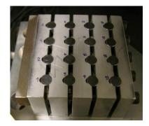
Figure 5: 16 capacitive sensors
