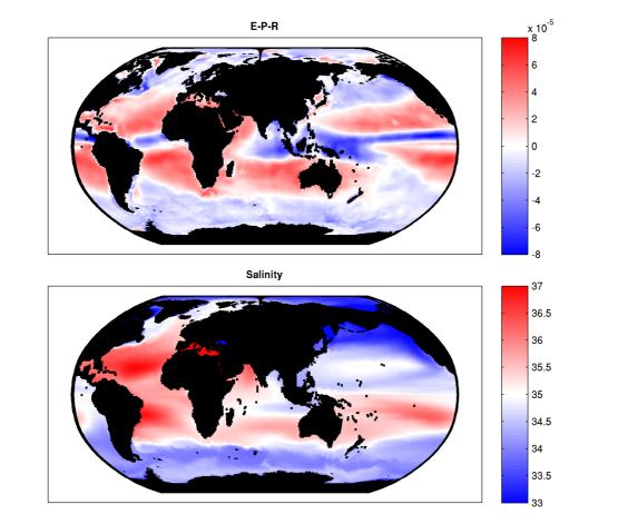
**Fig. 1.** Top panel: evaporation-precipitation-runoff flux for the global ORCA12 model  $(kgm^{-2}s^{-1})$ . Positive values correspond to regions where evaporation is dominant. Bottom panel: salinity (PSU) averaged over the top 200 m in the ORCA12 model. It is a time-mean over the last 10 yr of a 85 yr long experiment.
