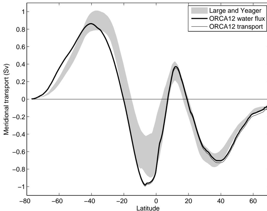
**Fig. 3.** Meridional transport resulting from the surface water flux in the ORCA12 model (Sv, thick black line), and comparison with Large and Yeager (2009). The grey shading is the envelope of all annual transports resulting from the air-sea fluxes of Large and Yeager (2009) for years 1984 to 2006 (these fluxes are a combination of observations and the NCEP reanalysis). The thin black line is the meridional transport computed directly from the model meridional velocities.
