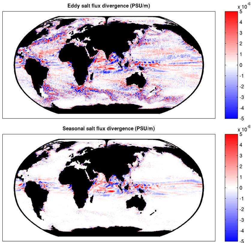
**Fig. 7.** Divergence of the eddy salt transport in the ORCA12 simulation, computed for  $12 \times 12$  grid point boxes to enhance readability. It is integrated vertically and thus expressed in units of  $\text{PSUms}^{-1}$ . The colorscale is saturated in the red and blue at  $5 \times 10^{-6} \text{PSUms}^{-1}$  (the maxima and minima of the field are about 40 times larger). Top panel: total eddy component; bottom panel: seasonal contribution only.
