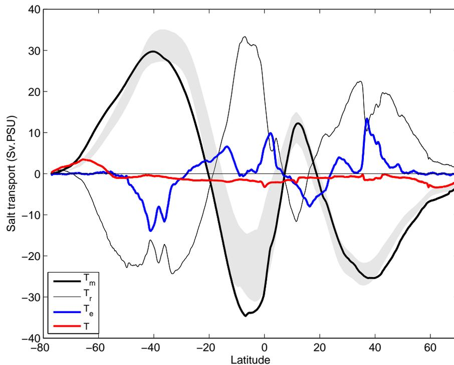
**Fig. 4.** Decomposition of the global meridional transport of salt in the ORCA12 simulation. See text (Eq. 8) for the explanation of the different terms. The grey shading is the observed salt flux carried by the net volume flux at each latitude: it is computed from the data of Large and Yeager (2009) (similar to Fig. 3) combined with the Levitus depth-averaged salinity field.
