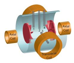
FIG. 1. (Color online) Schematic of the experimental setup, in flow configuration 2 (see text for details). Probe shafts represent the location of the magnetic field sensor arrays.
