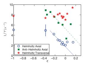
FIG. 3. (Color online) Evolution of relaxation decay time from an applied Helmholtz axial magnetic field (open blue circles), having an m=0 dipolar structure, an applied anti-Helmholtz axial magnetic field (green squares), having an m=0 quadrupolar structure, and an applied Helmholtz transverse magnetic field (red stars), having an m=1 dipolar structure, as a function of  $\epsilon$ . The lines are the linear extrapolation of the  $1/\tau$  evolution in the range  $-0.3 < \epsilon < 0$ .
