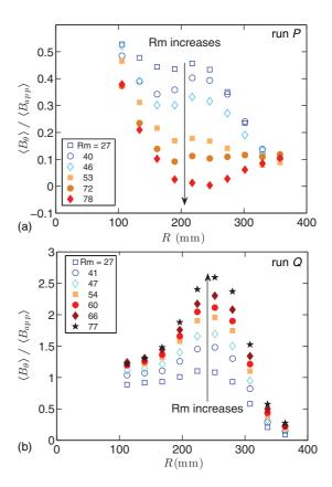
FIG. 9. (Color online) Normalized induced azimuthal magnetic field radial profile in probe shafts closer to one impeller as function of Rm for (a) run P, (b) run Q.
