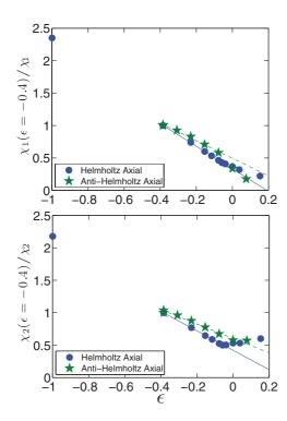
FIG. 5. (Color online)  $1/\chi$  as a function of  $\epsilon$  for the dynamo run, Helmholtz axial, and anti-Helmholtz axial setups. Curves have been normalized to their values at  $\epsilon = -0.4$ ; see text for detailed definitions of  $\chi_1$  and  $\chi_2$ . Linear fits (in the range  $-0.4 < \epsilon < 0$ ) shown as full and dashed lines.
