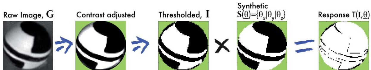
FIG. 4. (Color online) Texture extraction and comparison with a synthetic image. The resemblance between the image \underline{\mathbf{I}} and the synthetic projection \underline{\mathbf{S}} at angle \theta is estimated using Eq. (13).
