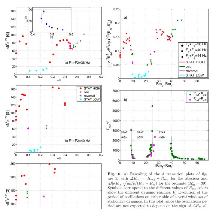
**Fig. 5.** (a) Transition plots as asymmetry  $(\theta)$  is varied at fixed F. a)  $F_1 + F_2 = 36$  Hz. Color code as in (b). The inset shows the corresponding evolution of the period of oscillation in the oscillating/reversing regimes. (b)  $F_1 + F_2 = 40$  Hz. (c)  $F_1 + F_2 = 44$  Hz. Color code as in (b).
