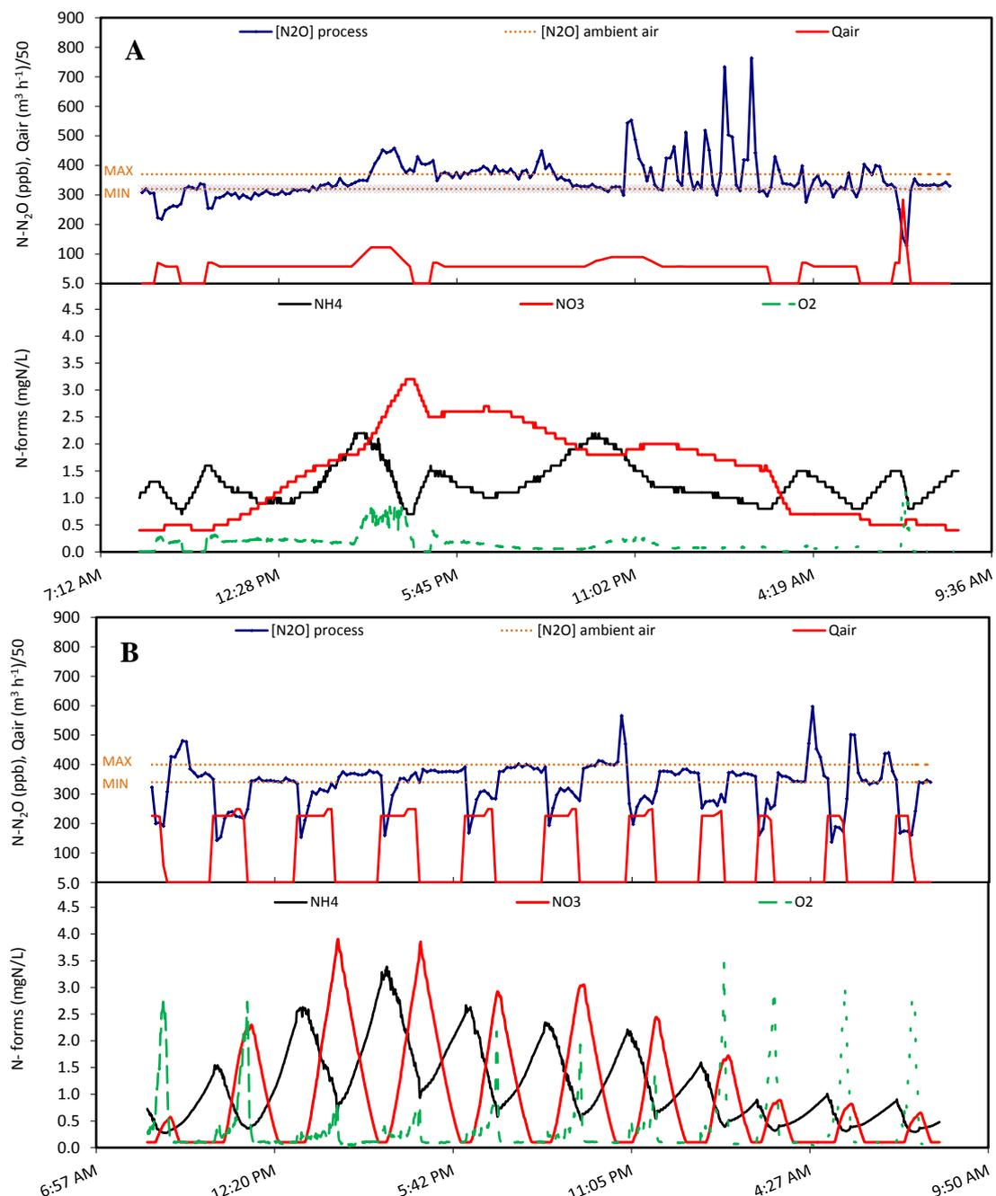
**Figure 2.** Off-gas N<sub>2</sub>O concentration, air flow and nitrogen forms concentration in tank 1 (A) and tank 2 (B) - aerated zones.
