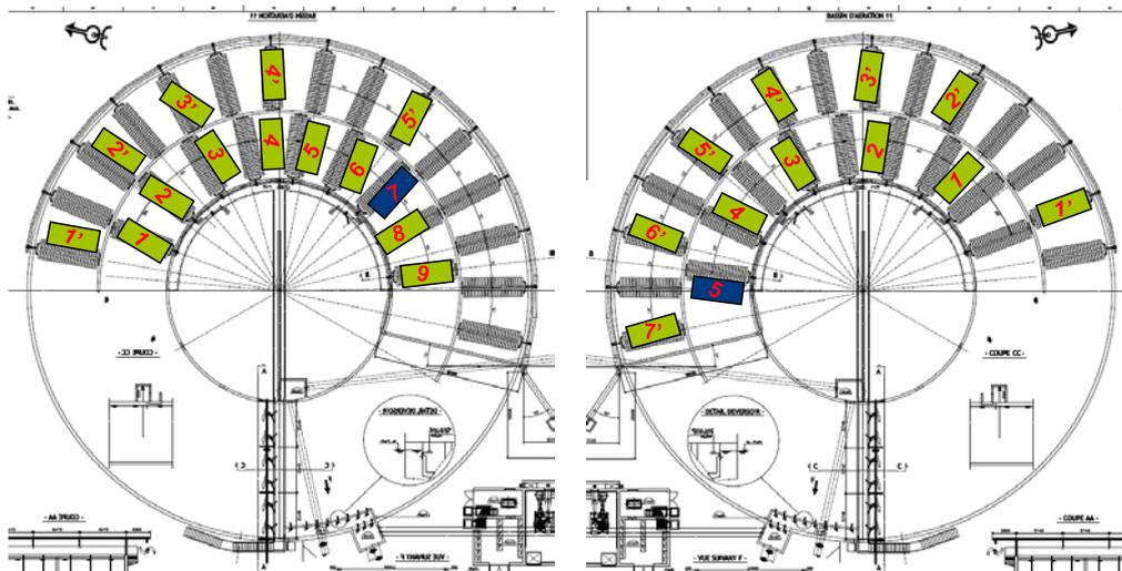
**Figure 1.** Sampling points for oxygen mass transfer measurement (■) and collectors position for the monitoring of N<sub>2</sub>O emissions (■) in tank 1 (right) and tank 2 (left)
