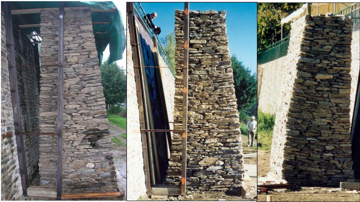
Fig. 7. Wall 5, left: before loading, centre and right: after loading “belly shape”.
