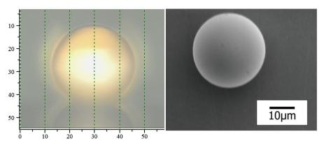
Fig. 3 Optical microscope and SEM image of  $Er^{3+}$ :  $Ga_5Ge_{20}Sb_{10}S_{65}$  micrometer microsphere coated with Au/Pd conductive layer at the surface for SEM imaging.
