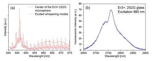
**Fig. 4** Feasibility investigation: (a) Raman and fluorescence spectra for 633 nm excitation in the center and border of an equatorial plane of the  $Er^{3+}$ :  $Ga_5Ge_{20}Sb_{10}S_{65}$  microsphere. (b) Fluorescence spectrum of  $Er^{3+}$ :  $Ga_5Ge_{20}Sb_{10}S_{65}$  glass excited at 980 nm.
