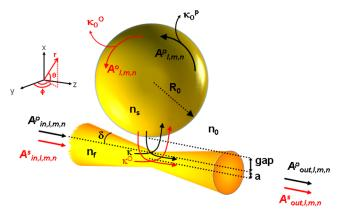
**Fig. 1** Layout sketch of the chalcogenide fiber taper coupled to the Er<sup>3+</sup>-doped chalcogenide microsphere.
