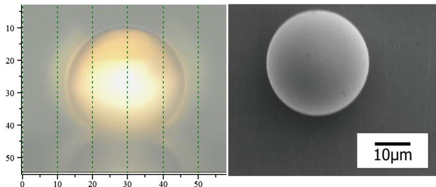
**Fig. 3** Optical microscope and SEM image of Er<sup>3+</sup>:Ga<sub>5</sub>Ge<sub>20</sub>Sb<sub>10</sub>S<sub>65</sub> micrometer microsphere coated with Au/Pd conductive layer at the surface for SEM imaging.
