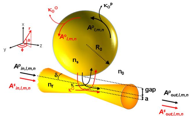
**Fig. 1** Layout sketch of the chalcogenide fiber taper coupled to the Er<sup>3+</sup>-doped chalcogenide microsphere.
