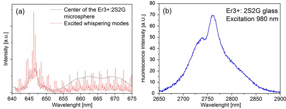
**Fig. 4** Feasibility investigation: (a) Raman and fluorescence spectra for 633 nm excitation in the center and border of an equatorial plane of the Er<sup>3+</sup>:Ga<sub>5</sub>Ge<sub>20</sub>Sb<sub>10</sub>S<sub>65</sub> microsphere. (b) Fluorescence spectrum of Er<sup>3+</sup>:Ga<sub>5</sub>Ge<sub>20</sub>Sb<sub>10</sub>S<sub>65</sub> glass excited at 980 nm.
