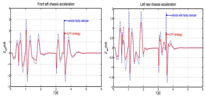
Fig. 18. Chassis acceleration in front left  $\ddot{z}_{s_{fl}}$ .
