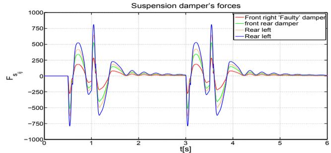
Fig. 4. Suspension damper's forces: the faulty and healthy dampers efforts
