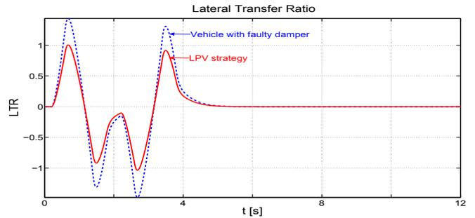
Fig. 3. Lateral load transfer
