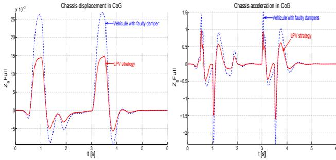
Fig. 6. Chassis displacement in CoG  $z_s$ .
