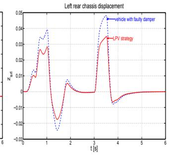
Fig. 15. Chassis displacement in rear left  $z_{s_{rl}}$ .
