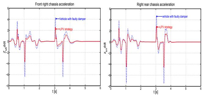
Fig. 16. Chassis acceleration in front right  $\ddot{z}_{s_{fr}}$ .
