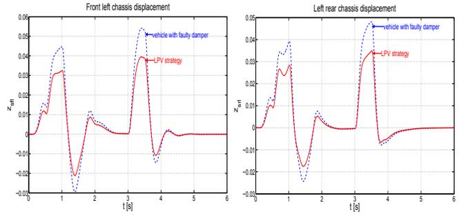
Fig. 14. Chassis displacement in front left  $z_{s_{fl}}$ .
