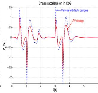
Fig. 7. Chassis acceleration in CoG  $\ddot{z}_s$ .
