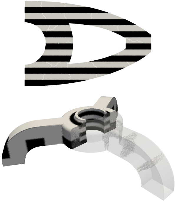
Figure 6: Tripod used for our 3D and cantilever used for our 2D strong scaling experiments. Black and light grey are used to represent the variations of the Young’s modulus (200 GPa and 0.01 GPa) and Poisson’s ratio (0.25 and 0.45).
