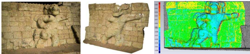
Figure 6: Examples of the geometric comparison with ground-truth data. Original scene (left), derived 3D point cloud (center) and deviation map for a Maya bas-relief (std = ca 5 mm).
