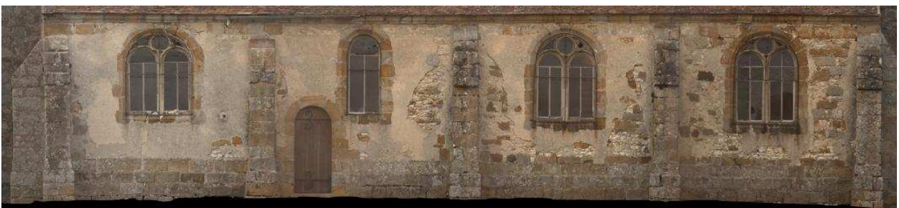
Figure 4: A typical orthoimage generated by orthographic projection of a dense point cloud.
