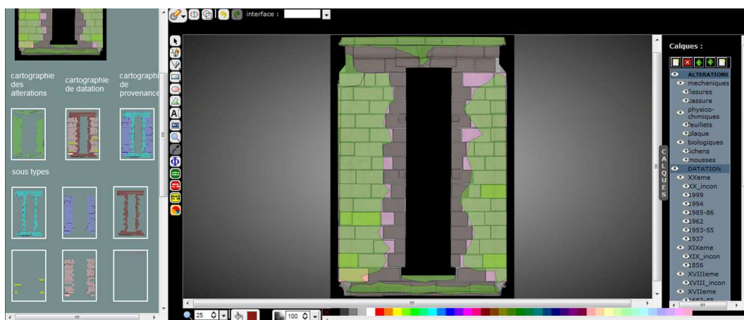
Figure 6. Interface implemented basing on svg-edit free editor according to conservation purposes. On the right, hierarchical layers concerning different cartography types.
