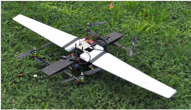
Fig. 4. Quad-plane experimental platform, developed at HEUDIASYC laboratory.
