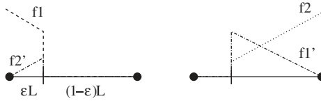
Figure 3. Truncated function basis for a 1D cracked element (shadow node version). This basis is equivalent to the one depicted in Figure 2.
