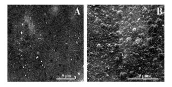
**Fig. 2.** SEM images of GC electrode surfaces before and after electrochemical reduction. DMF + 0.1M TBABF<sub>4</sub>. (A)—Initial GC surface. (B)—Blank experiment on the same GC sample with a hold of potential at -2.5 V during 5 min.
