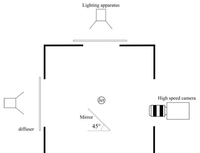
**Figure 4:** Sketch of the experimental set-up.
