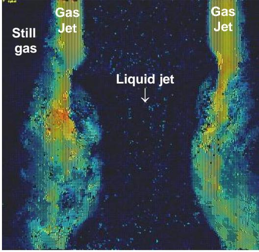
**Figure 11:** PIV visualization of gas flow around the liquid flow: non axi-symmetric KH wave induce non-axisymmetric recirculations.
