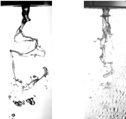
**Figure 1:** Instability of a liquid jet in airblast atomization for: a)  $U_g = 14$  m/s,  $U_l = 0.25$  m/s; b)  $U_g = 18.7$  m/s,  $U_l = 0.31$  m/s. a) KH wave is non-axisymmetric ; b) KH wave is axisymmetric.
