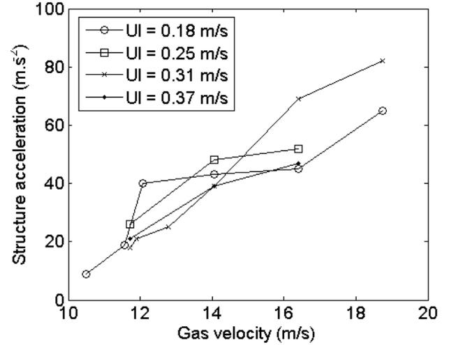
**Figure 12:** Acceleration of the liquid structure with gas and liquid velocity.
