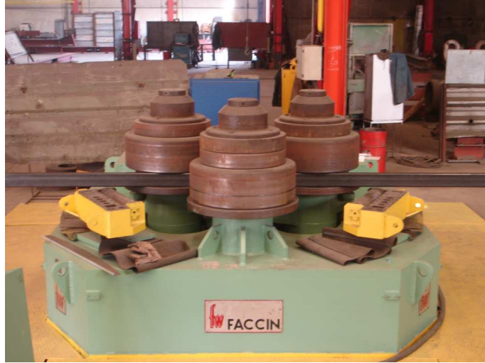
Figure 2: Example of cold curving machine (courtesy EMEK S.A., Greece)
