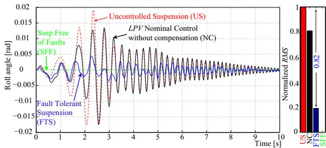
Fig. 4. Performance of the *FTC* in the test #1 (left) and comparison w.r.t. the uncontrolled suspension by using a normalized *RMS* (right).
