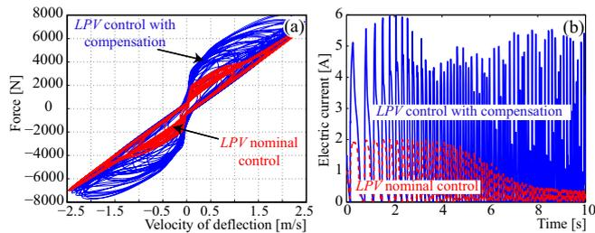
Fig. 5. Semi-active damping force in the front-right corner with and without fault compensation (a), and the corresponding controller output (b).
