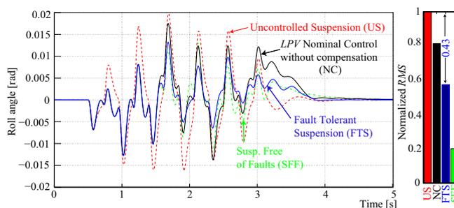
Fig. 6. Performance of the *FTC* in the test #2 (left) and comparison w.r.t. the uncontrolled suspension by using a normalized *RMS* (right).
