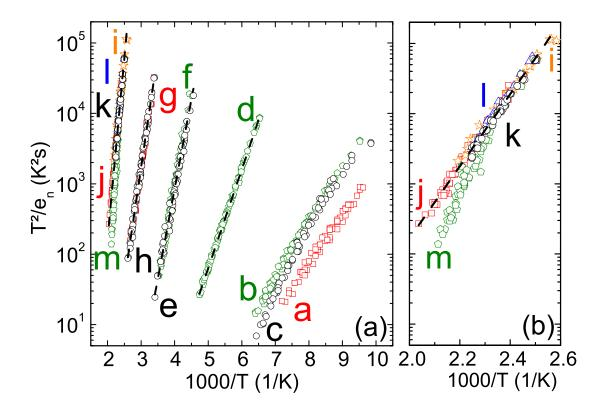
FIG. 2. (a) Arrhenius diagram of levels measured by Fourier transform deep level transient spectroscopy in five n-type ZnO samples. A letter label is attributed to each level. (b) Same as (a) but focused on the [E1000] level. Data coming from sample #1 are represented in open squares, #2 in open circles, #3 in open stars, #4 in open pentagons, #5 in open triangles and dash lines correspond to the linear fit of data.
